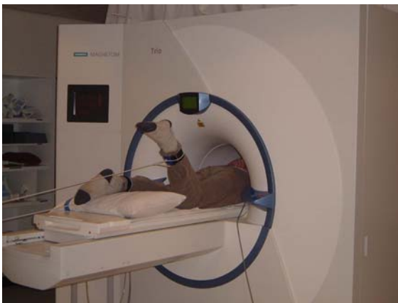
Fig. 1 The experimental set-up for prone dynamic exercise ^{31}\text{P} spectroscopy at 3 Tesla. Subjects were requested to perform alternate knee flexion with 0.5 kg leg weights attached to each ankle. Haemodynamic measurements of pulse, blood pressure, oxygen saturations were made continuously
